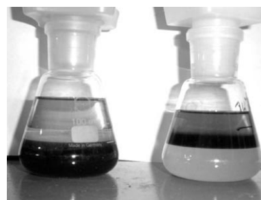
Figure 9. Phase separation of the aqueous biphasic 1-octene hydroformylation mixture in the presence of block copolymer P2 (left) and the random copolymer P1 (right).
